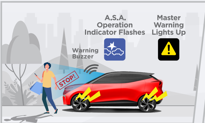
Warning buzzer + secondary brake (strong)
