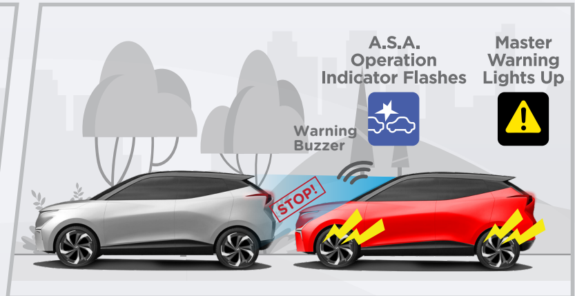
Warning buzzer + secondary brake (strong)
