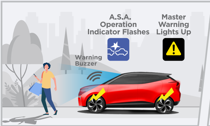
Warning buzzer + primary brake (weak)
