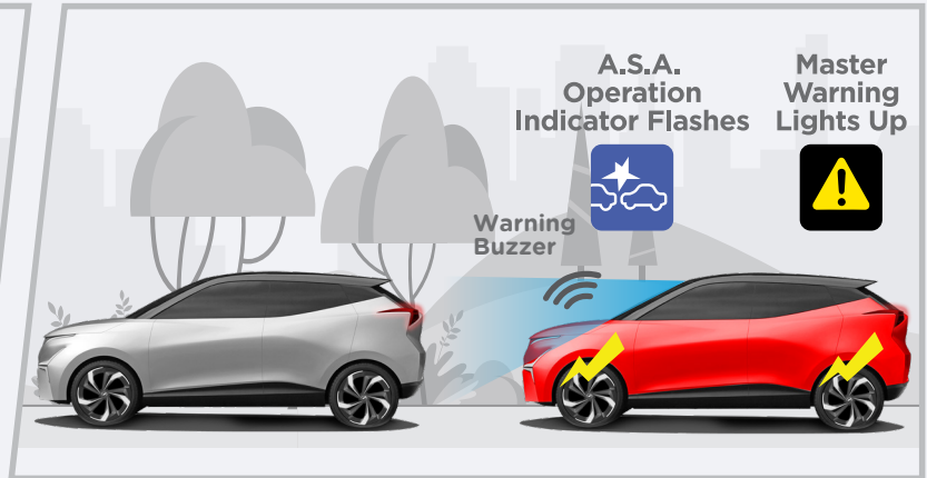
Warning buzzer + primary brake (weak)
